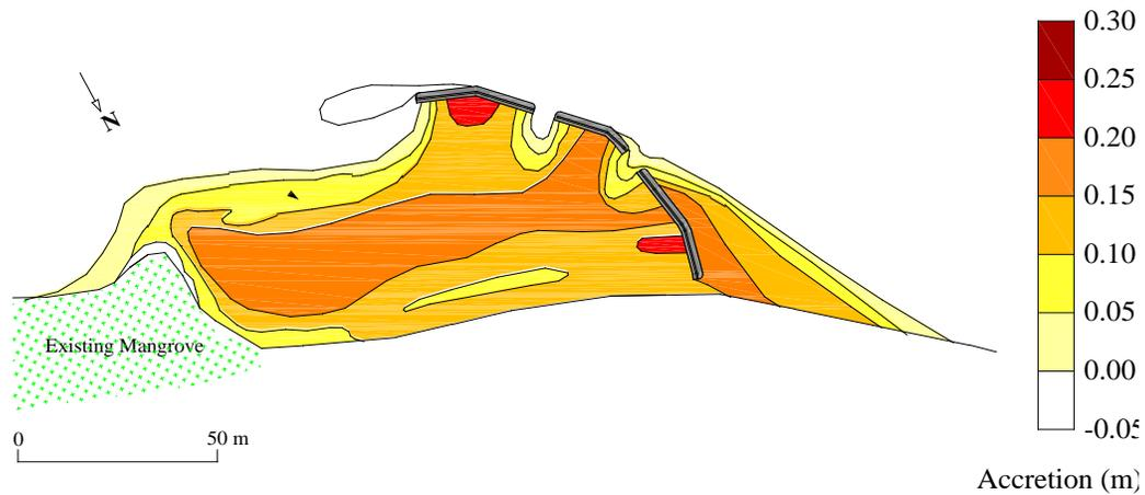
**Fig 7.a.** Rate of Sediment accretion at the mangrove plantation site in February 2009, 8<sup>th</sup> month after construction of L Block Break
