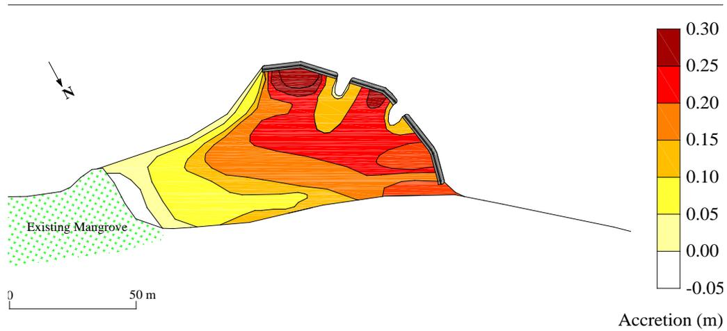
**Fig 7.** Rate of Sediment accretion at the mangrove plantation site in October 2008, 4<sup>th</sup> month after construction of L Block Break water
