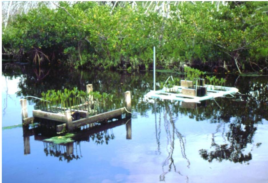
Fig. 3. In the field experiments, fixed and floating nurseries of planted red mangrove seedlings were monitored for plant growth and survival in controlled impoundments and open bay sites.
